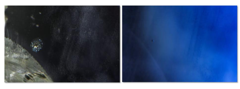
After heating with pressure: Improvement in clarity due to the healing of the narrow-gap fissure at lower left and the halo around the crystal inclusion.
