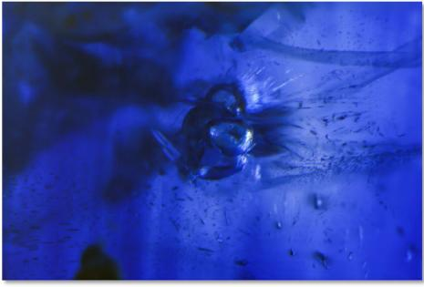
After heating with pressure: Typical damage from high temperature heat treatment, also a great improvement of colour.
