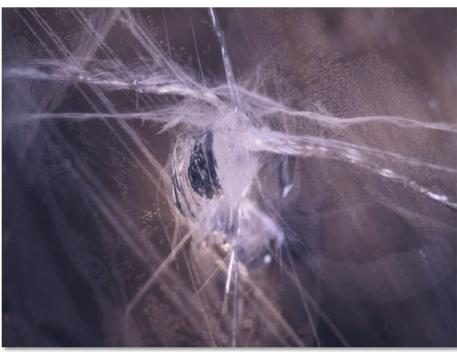
After heating with pressure: Serious deterioration of clarity with new fissures resulting from the treatment.
