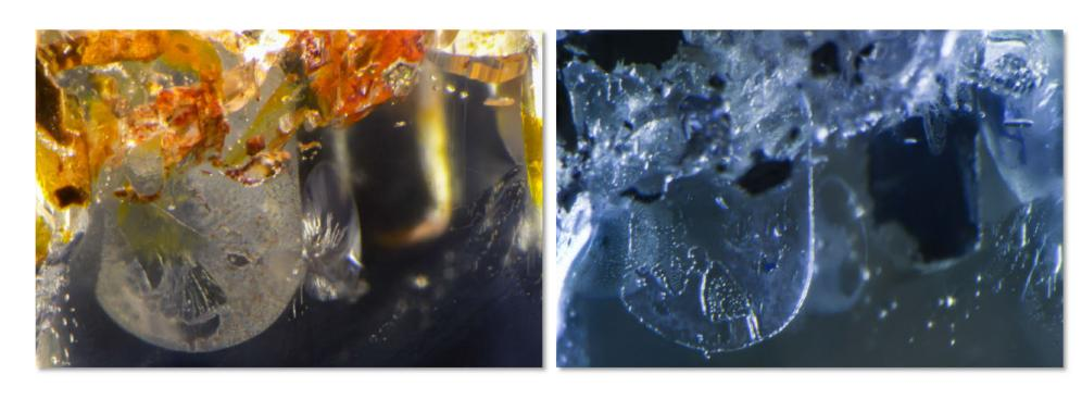
After heating with pressure: Iron staining gone, fissure in the middle partially healed but still quite visible.
