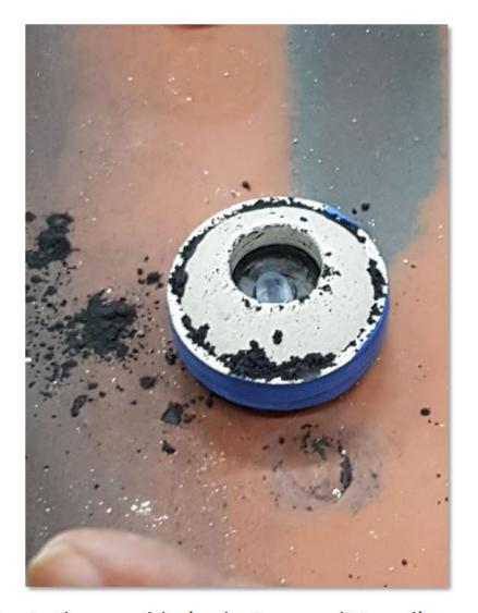
Graphite is packed around the sapphire in the crucible (reducing conditions!)
