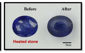
Examples of samples before and after heating with pressure
