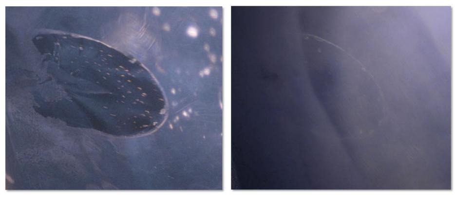
After heating with pressure: Improvement in clarity due to the healing of a narrow-gap fissure.
